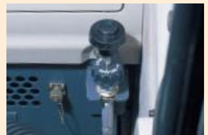
Emergency throttle cable
